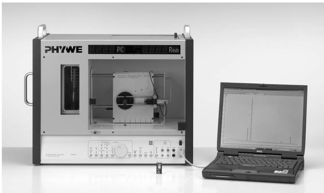
Figure 1. The x-ray diffractometer to be used in this experiment
