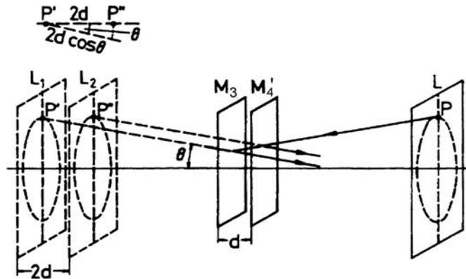
Figure 2. Formation of circular interference fringes.
