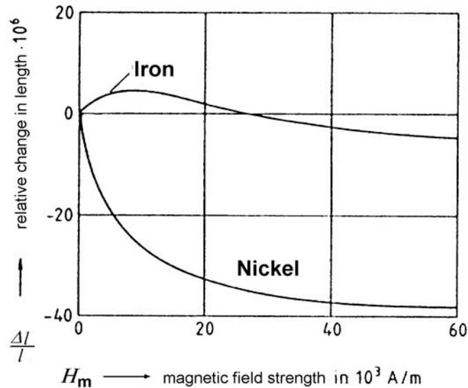
Figure 4. Magnetostriction of different ferromagnetic materials with their relative change in length  $\Delta l/l$  plotted against applied magnetic field strength  $H_m$ .
