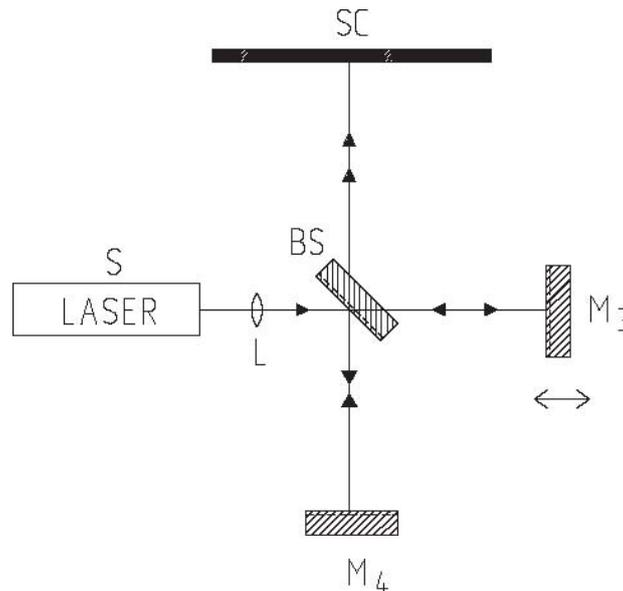
Figure 1. Michelson arrangement for Interference. S represents the light source; SC the screen.
