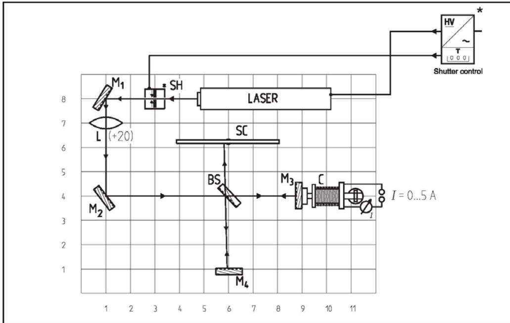
Figure 3. Schematic of the experimental set-up of the Michelson interferometer for the measurement of magnetostriction of different ferromagnetic materials. Note the shutter is not used in this experiment.
