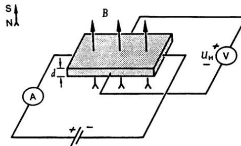
Figure 2. Schematic of the Hall effect.
