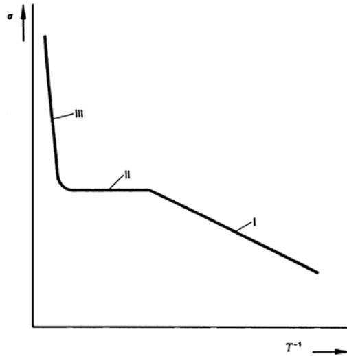
Figure 1. Conductivity of an ideal semi-conductor as a function of the reciprocal of the temperature
