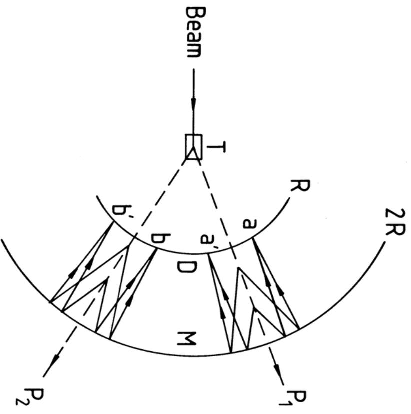
**Fig 4.11** Two particles  $P_1$  and  $P_2$ , emitted from the target T, emit Cerenkov radiation on traversing a medium contained between two spheres of radius R and 2R. The mirror M on the outer sphere focuses the radiation into ring images at  $aa'$  and  $bb'$  on the inner detector sphere D. The radii of the ring images depend on the angle of emission of the Cerenkov radiation and hence on the velocities of the particles.
