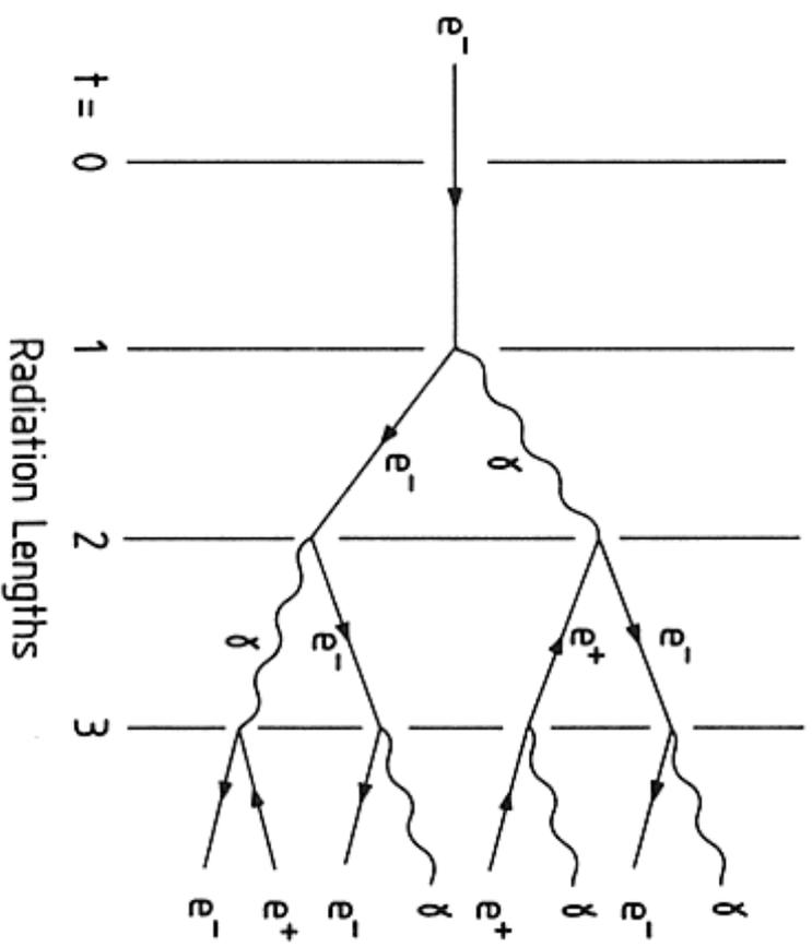
Fig.4.13 Simple model for the development of an electromagnetic shower
