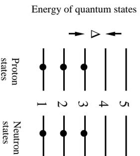
**Fig.2.5** Schematic diagram of nuclear energy levels near the highest filled levels. (In an actual nucleus the levels are not equally spaced.)
