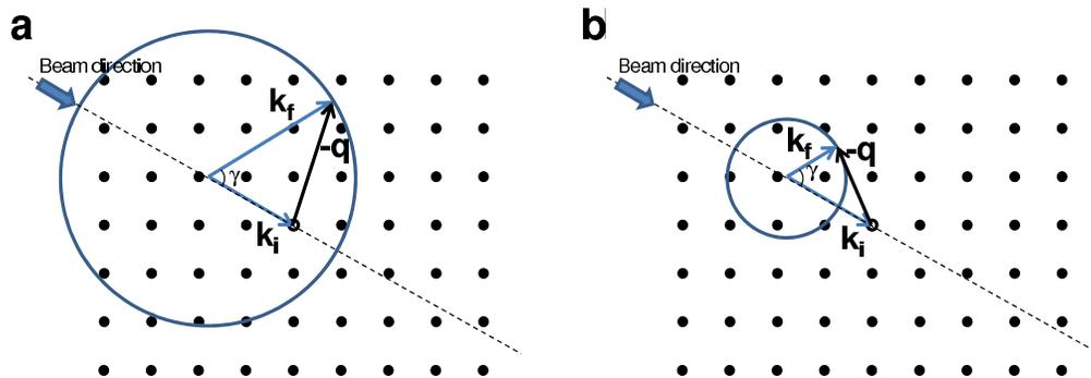
Figure 4: The procedure to construct the scattering triangle for inelastic scattering. (a) energy gain; (b) energy loss.
