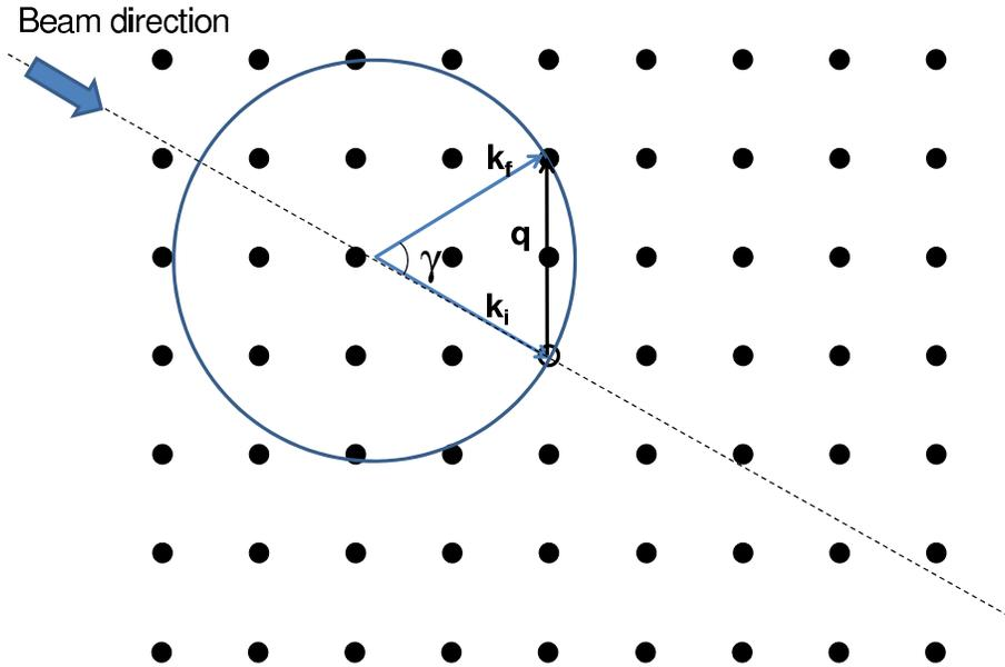
Figure 2: The procedure to construct the scattering triangle for elastic scattering.
