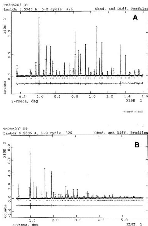
Figure 8: X-ray and neutron high-resolution powder diffraction at a glance. **A**: neutron powder diffraction (D2B-ILL, Grenoble, France,  $\lambda = 1.594$ ) and **B** synchrotron x-ray diffraction (X7a-NSLS, Brookhaven, USA,  $\lambda = 0.5000$ ) data on the pyrochlore compound  $\text{Tl}_2\text{Mn}_2\text{O}_7$ . Both data sets are fitted using the **Rietveld method** (see lecture and extended lecture notes)
