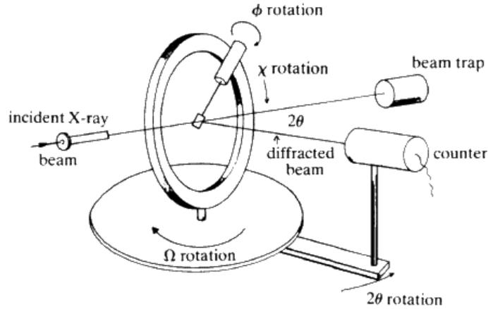
Figure 3: The geometry of a “four circle” single-crystal diffractometer. The “four circles” (actually four axes) are marked “ $\phi$ ”, “ $\chi$ ”, “ $\Omega$ ” and “ $2\theta$ ”. The  $2\theta$  and  $\Omega$  angles are also known as  $\gamma$  and  $\eta$  — a notation we will often employ in the remainder to avoid clutter and confusion with other symbols (e.g., the solid angle)
