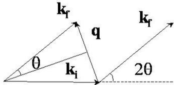
Figure 1: Scattering triangle for elastic scattering.
